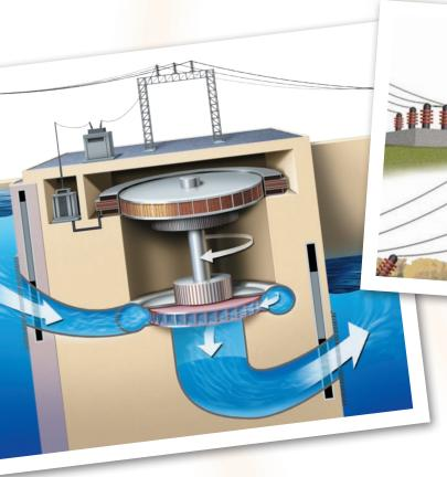
Inside a hydroelectric [hy•droh•ee•LEK•trik] dam, the mechanical energy of falling water is used to turn generators, which change mechanical energy into electrical energy. Electricity generating stations, also know as energy stations, may use water, coal, or atoms to produce the electricity you use.
